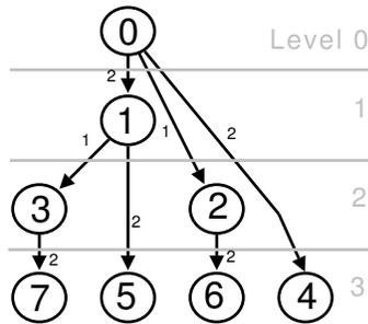
Fig. 10. Binomial tree pattern with 8 processes annotated with the maximum congestion along each path.
