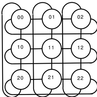
Fig. 14. 3-ary 2-cube network with endpoint numbering.
