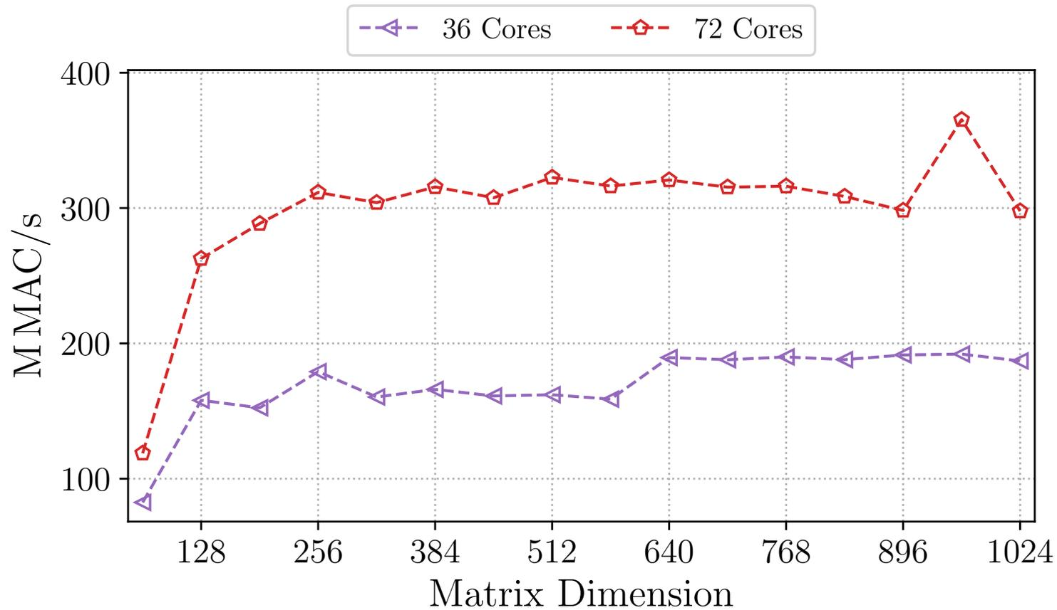
Xilinx Alveo U250 vs. CPU nodes with 2× Intel Xeon E5-2695 v4
