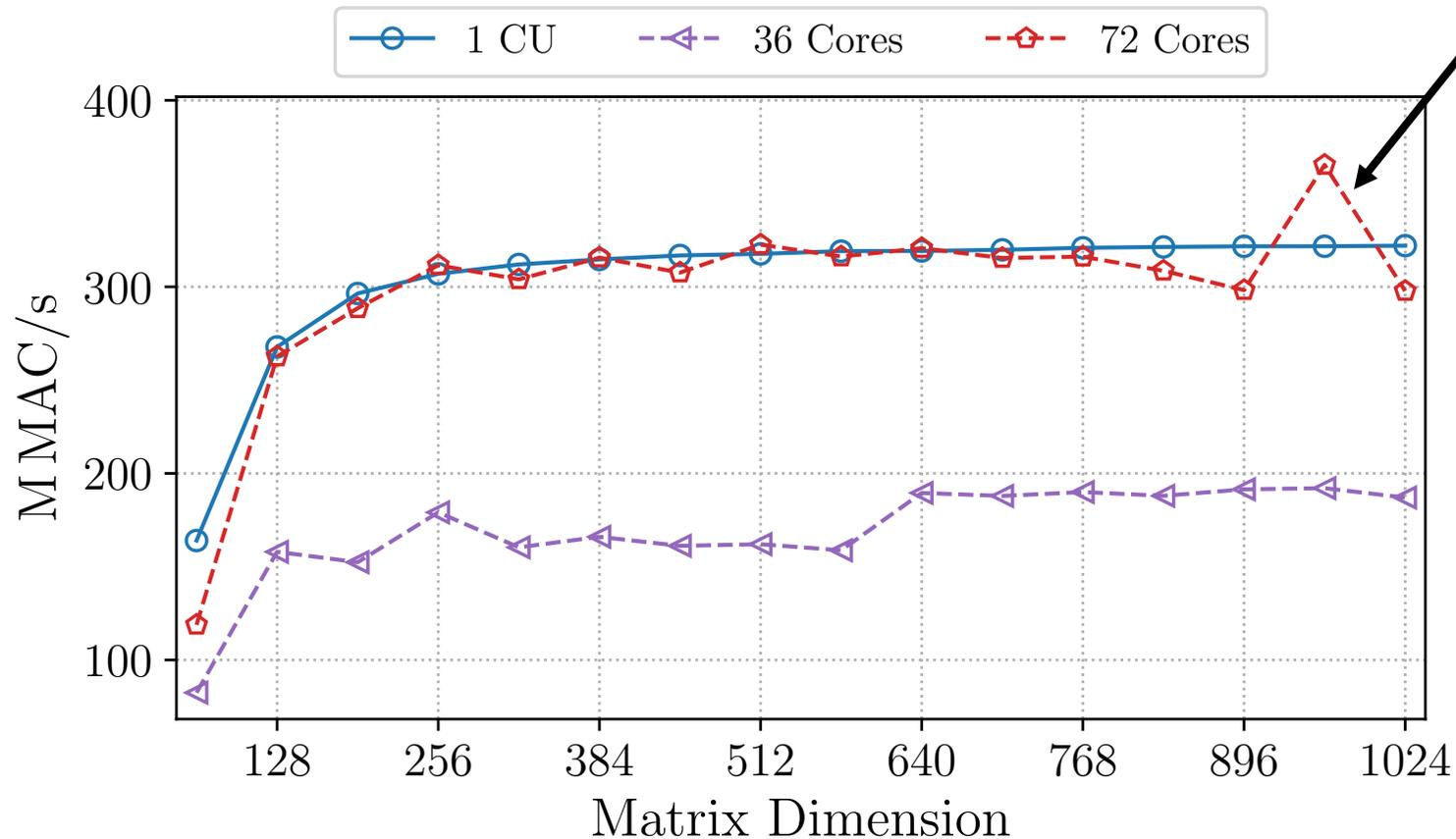
Xilinx Alveo U250 vs. CPU nodes with 2x Intel Xeon E5-2695 v4
