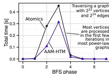
Figure 1: Comparison of the duration of an intra-node BFS traversal implemented with Blue Gene/Q fine-grained atomics and coarse hardware transactions (AAM-HTM). One transaction modifies  $2^7$  vertices. We use 64 threads and a Kronecker graph [23] with a power-law vertex degree distribution.
